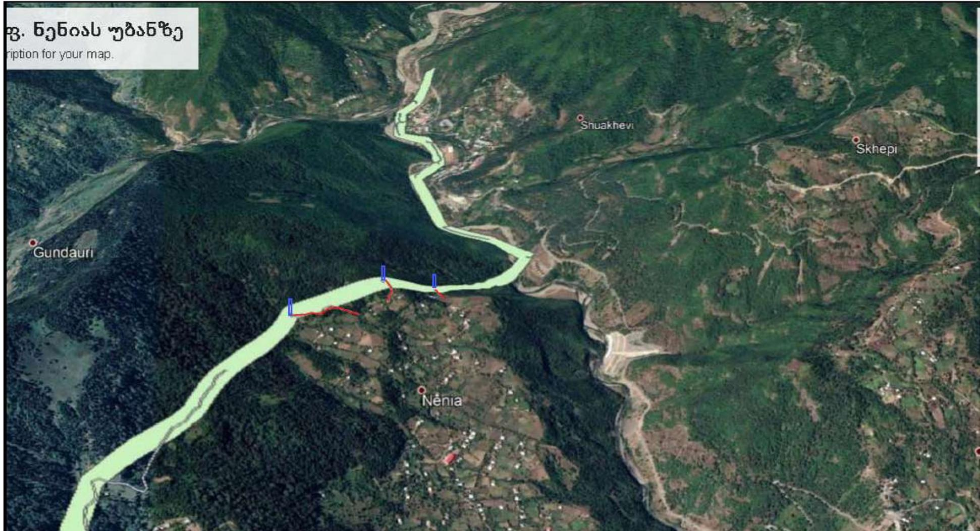
Fig.: three towers (blue posts) and access roads (red lines) near Village Nenia.
