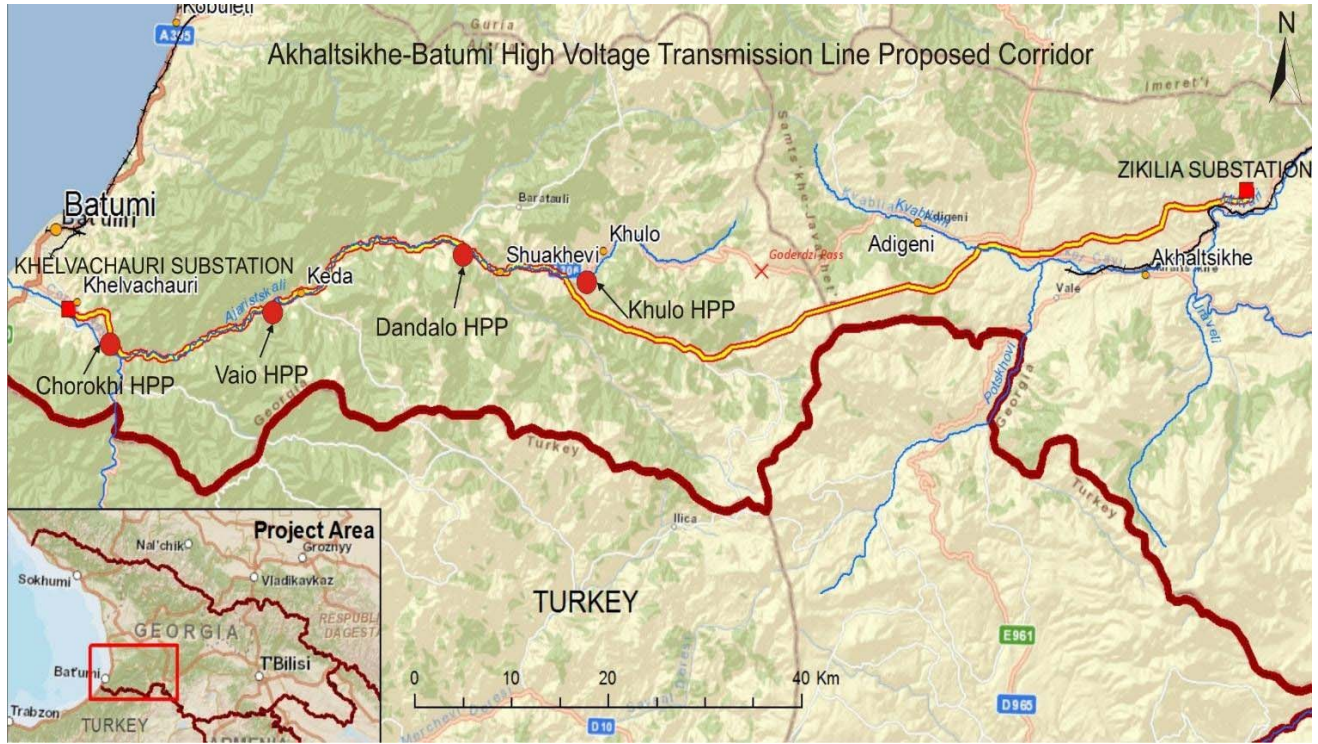
Fig.1.1 Entire alignment of the 220kV OHL from Akhaltsikhe 500/400kV Back to Back substation to Batumi 220kV substation
